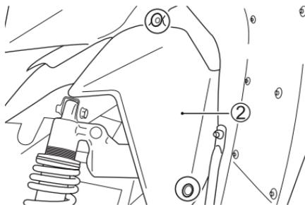
3. Remove the fasteners and cover ②.
